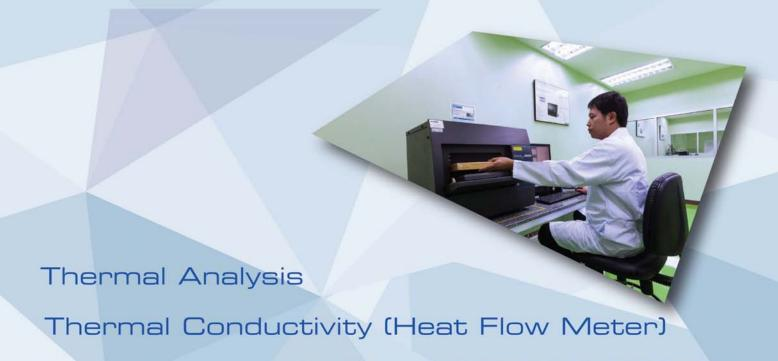
This instrument works according to well-established standards: ISO 8301, ASTM C518, EN12667 and EN 13939. It comes with a traceable calibration standard. Heat flow meter systems can be employed for the measurement of thermal conductivity and/or thermal resistance of insulation material. (Ref. www.netzsch-thermal-analysis.com)
