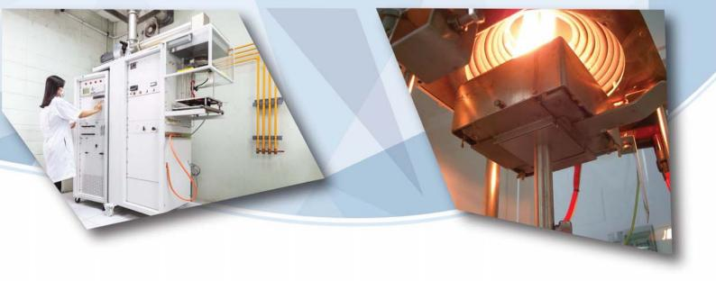
We also have the reliable testing instruments such as Cone calorimeter, derived from Fire Testing Technology (FTT) in UK which the largest and leading manufacturer of Cone calorimeter. The Cone calorimeter is the most significant bench scale instrument in the field of fire testing. Directly measured properties include:
